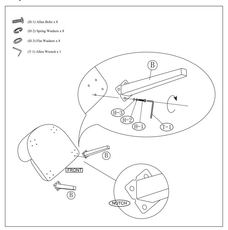
Lay the Chair Seat(A) upside down on a padded non-marrying surface. Open the leg box packaging and remove both Front Legs(B) and Rear Legs(C). First, install Front Legs(B) at the front of Chair Seat(A). Secure using Allen Bolts (H-1). Spring Washers(H-2) and Flat Washers(H-3), stacking the hardware in the order as shown. Fully tighten all bolts using Allen Wrench (T-1). Please note the notches in the metal leg plate should all face toward the center of the chair.
