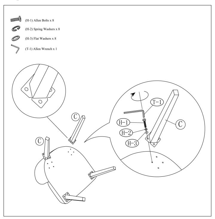
Next, install Rear Legs(C) and secure using Allen Bolts(H-1). Spring Washers(H-2) and Flat Washers(H-3), stacking the hardware in the order as shown. Fully tighten all bolts using Allen Wrench(T-1). Please note the notches in the metal leg plate should all face toward the center of the chair.
